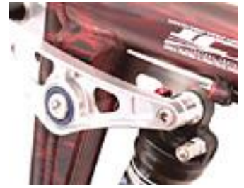
Trick new CNC upper rocker arm
