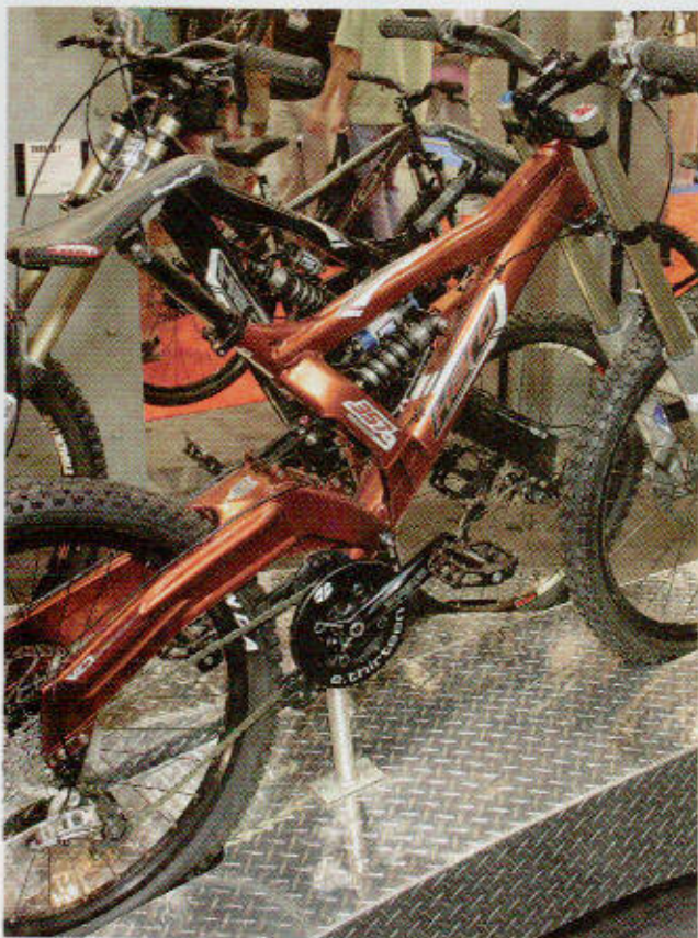
Haro 357: Another rule-breaker from Haro, the 357 Magnum downhill chassis squeezes the most from a single-pivot suspension.
