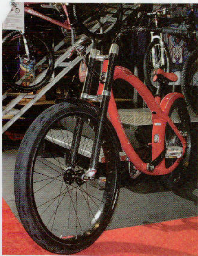
Breaking tradition: Tony Ellsworth designed a "performance-oriented" city cruiser around NuVinci's variable-speed hub transmission. The "Ride" is also cog-belt driven, so there is no messy chain to deal with.
