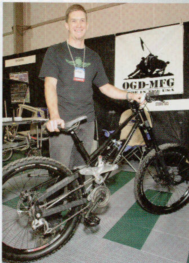
Torque control: ODG Manufacturing followed in the footsteps of Balfa Cycles by using an idler wheel above the chainring to prevent chain tension from affecting the rear suspension. (720) 352-3631.
