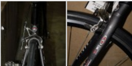
Another look at the rear end monostay Easton provided the carbon fiber rear triangle
