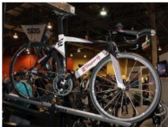
The new Ellsworth Coefficient carbon fiber time trial bike features front and rear wheel cutouts and aero-profile tubing.
